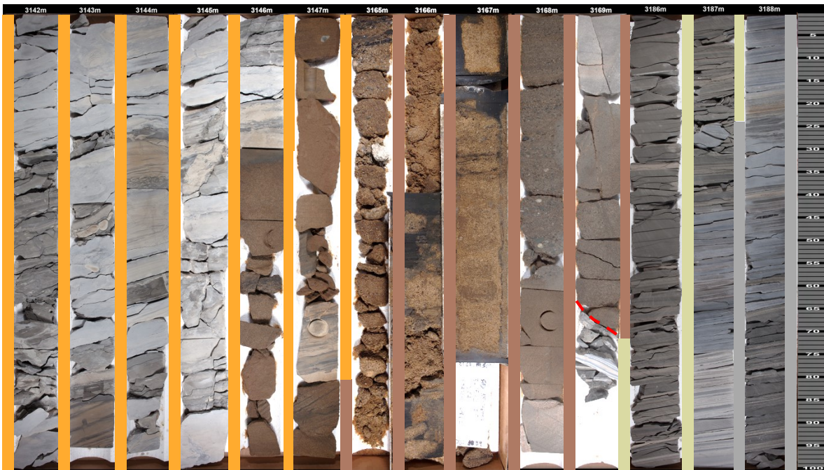
Figure 2.26 Bay du Nord (Bay du Nord member) L-76Z Core with DSE Selected core images, amongst cores 3 and 4, from Bay du Nord L-76Z. Colours represent depositional sub-environments; shelf (grey), incised valley (light brown), bay head delta (orange). Note the sharp basal Bay du Nord member contact denoted in a dashed red line.
